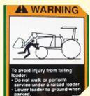
DO NOT WORK BENEATH BUCKETS OR RAISED LOADS. USE SAFETY PROP RODS DURING MAINTENANCE.
