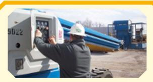
MACHINE OPERATORS MUST KNOW THE EMERGENCY CONTROLS OF THE MACHINE THEY'RE USING.
